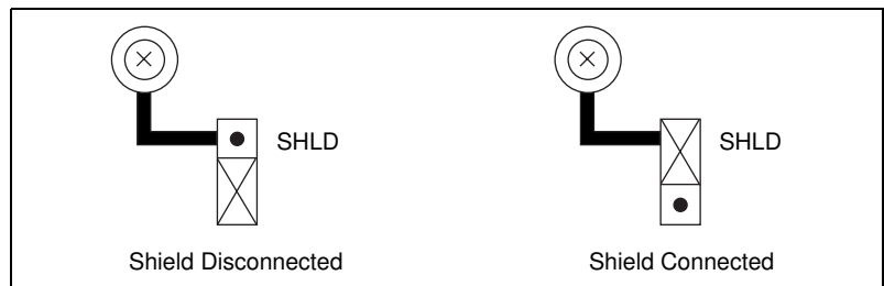
Figure 10-4. Ground Settings for Jumper W1
