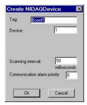
**Device** is the NI-DAQ device number. The DAQ configuration utility (WDAQConf.exe) assigns this number to an installed device. Valid device numbers range is from 1 to 16.
