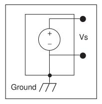
Figure 5-2. Grounded Signal Sources
