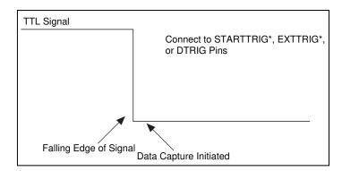
Figure 8-1. Diagram of a Digital Trigger
