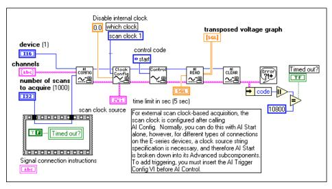
Figure 9-6. Externally Controlling Your Scan Clock with the Getting Started
