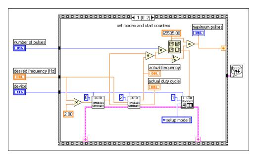
Figure 24-24. Frame 1 of Finite Pulse Train (8253) VI
