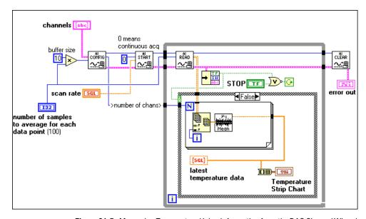
Figure 21-5. Measuring Temperature Using Information from the DAQ Channel Wizard
