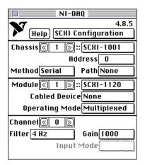
Figure 2-7. SCXI Configuration Window in NI-DAQ
