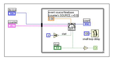
Figure 27-5. Diagram of Count Events-Easy (DAQ-STC) VI
