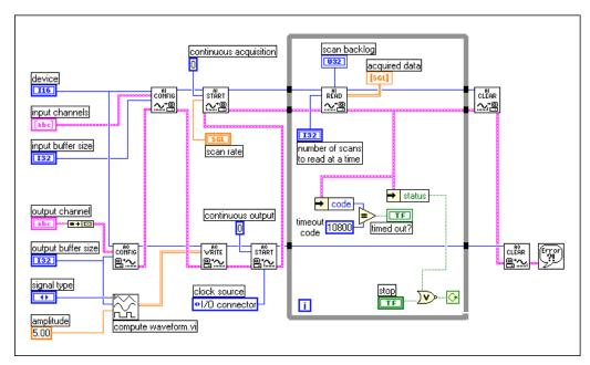
Figure 14-3. Simultaneous Input/Output Using the Simul Al/AO Buffered (Legacy MIO) VI
