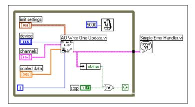
Figure 11-4. Multiple Immediate Updates Using Intermediate VI
