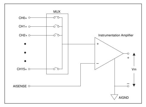
Figure 5-10. 16-Channel NRSE Measurement System
