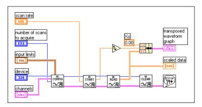
**Figure 7-6.** Simple Buffered Analog Input with Graphing
