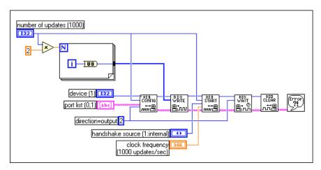
**Figure 17-5.** Pattern Generation Using the DIO-32 Series Devices
