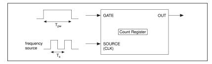
Figure 25-1. Counting Input Signals to Determine Pulse Width
