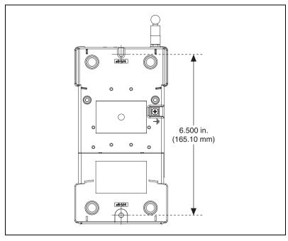
Figure 5. Device Panel Mounting Dimensions
