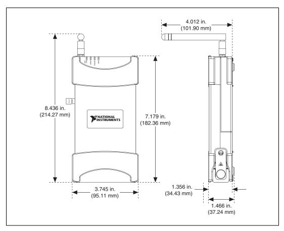
Figure 2 shows the NI WLS/ENET-9000 Series device dimensions.
