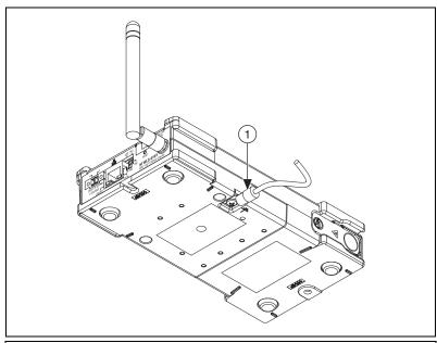
1 Ring Lug Attached to the Ground Screw
