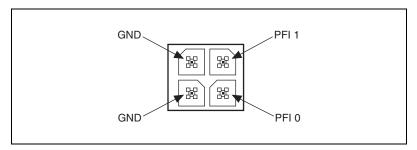
Figure 8. Trigger Connector Pinout
