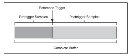
**Figure 10.** Reference Trigger Final Buffer
