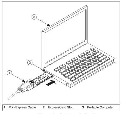
Figure 2-2. Installing the NI ExpressCard-8360
