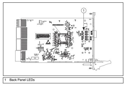
Figure 6. NI PXIe-8360 Back Side LED Locations
