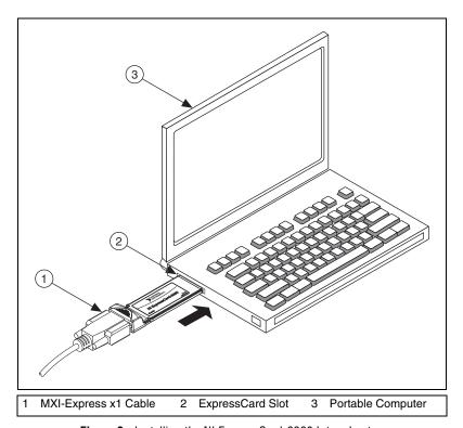
Figure 3. Installing the NI ExpressCard-8360 Into a Laptop
