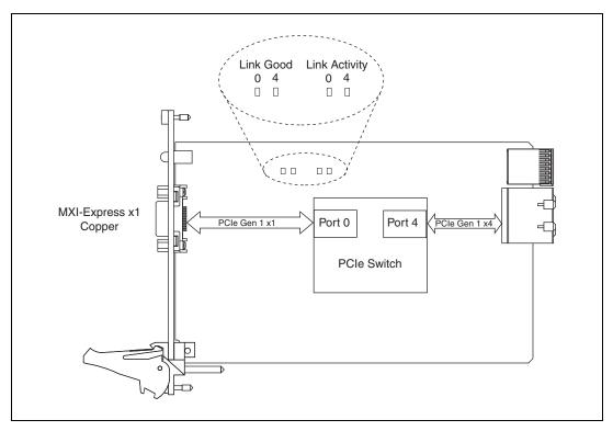
Figure 5. NI PXIe-8364 (193970x-01L) Onboard LED Locations
