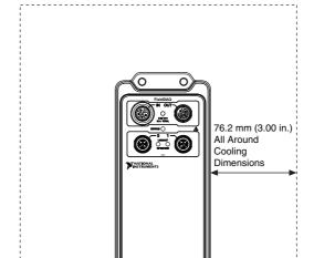
Figure 25. Cooling Dimensions
