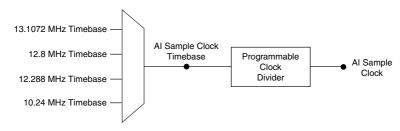
The FD-11603 is considered a Delta-Sigma device; it contains multiple A/D converters that require a high-frequency oversample clock to produce accurate, synchronized data. The FieldDAQ device returns a sample on every Sample Clock pulse.
