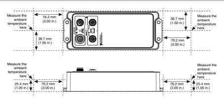
Figure 28. Ambient Temperature Locations, Vertical Mounting Configuration
