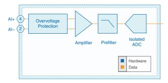
Figure 9. FD-11603 Block Diagram
