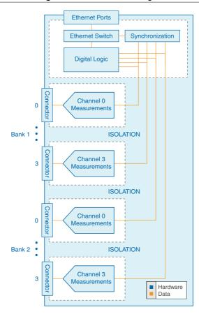
The FD-11603 provides channel-to-channel isolation. Input signals on each channel are conditioned, buffered, and then sampled by an ADC. Each AI channel provides an
