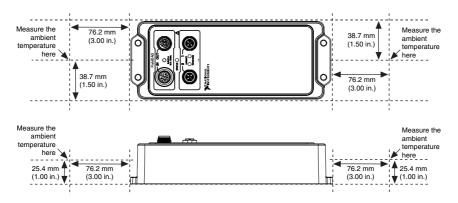
Figure 27. Ambient Temperature Locations. Vertical Mounting Configuration
