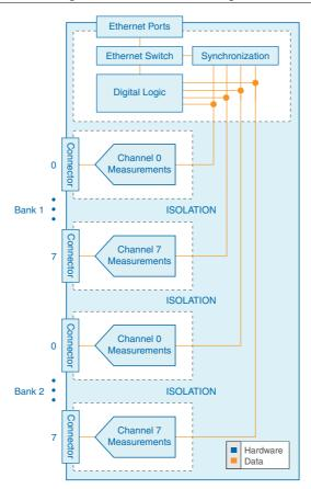
The FD-11614 provides channel-to-channel isolation.
