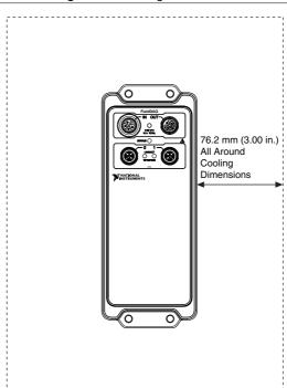
Figure 24. Cooling Dimensions
