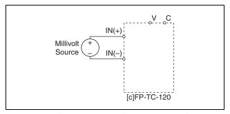
Figure 4. Connecting a Millivolt Source to the [c]FP-TC-120
