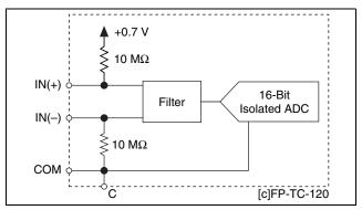
Figure 3. [c]FP-TC-120 Analog Input Circuitry on One Channel
