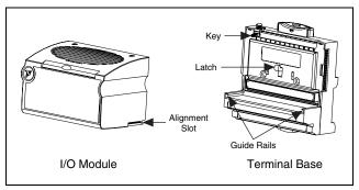
Figure 1. Installing the FP-TC-120
