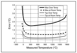
Figure 6. Type R and S Errors
