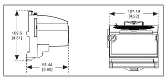
Figure 10. FP-TC-120 Mechanical Dimensions
