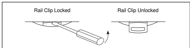
**Figure 2-1.** DIN Rail Clip in the Unlocked Position
