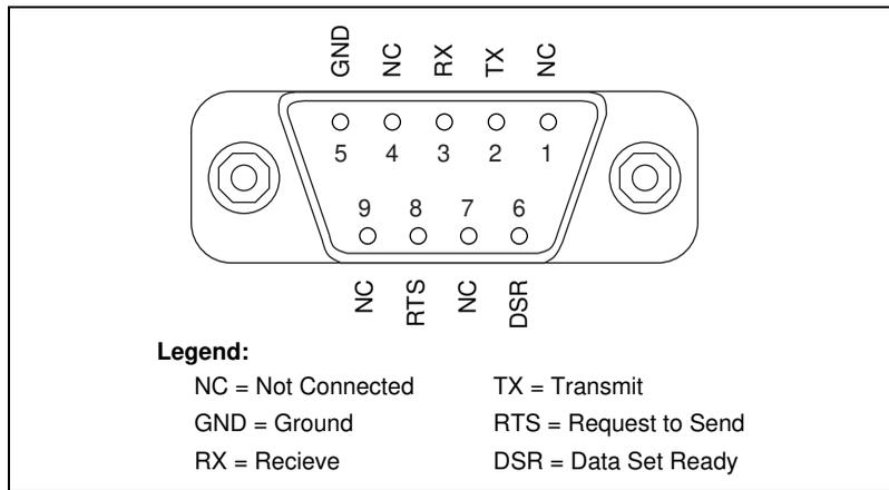
**Figure 2-9.** RS-232 Connector Pinout for the FP-1000
