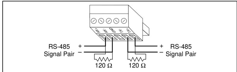
**Figure 2-12.** Terminating RS-485 Using the Combicon Adapter
