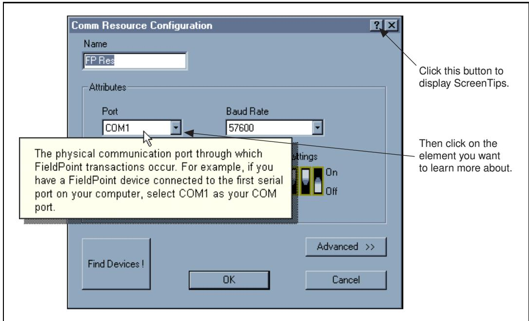
**Figure 4-3.** ScreenTips Showing a Description of an Item
