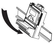
C. Slide base into position and lock rail clip. Be careful not to bend any pins.
