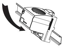
C. Slide module into position and lock rail clip.
