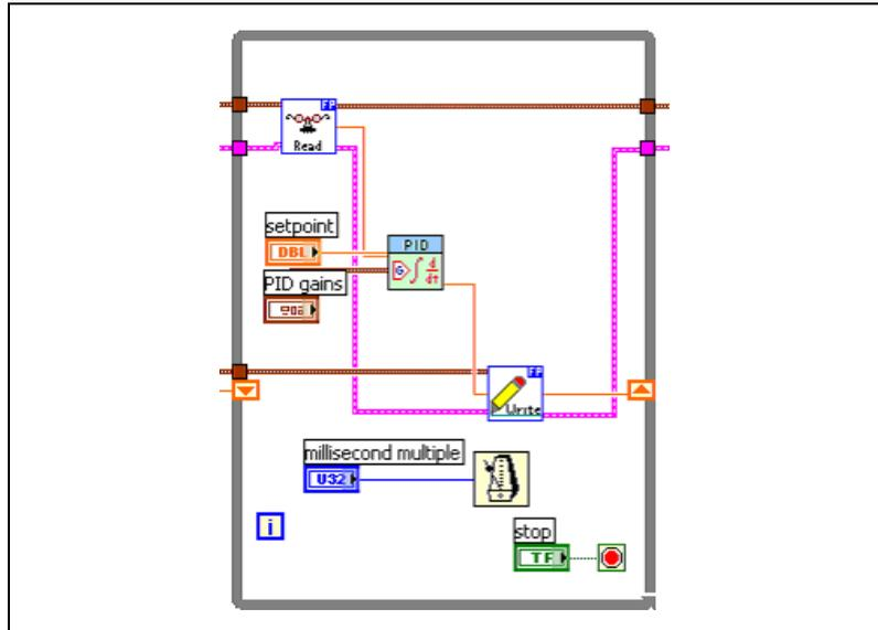
Figure 5-14. One Channel PID Output Using FieldPoint
