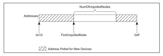
In other words, FirstUnpolledNode tells the LAS the beginning of a region of addresses to not probe, and NumOfUnpolledNodes tells the LAS the length of that region. So if FirstUnpolledNode were 0x25, and NumOfUnpolledNodes were 0xba, then no addresses from 0x25 to 0xdf would be probed. That means that if a device with an address of 0x25 were placed on this bus, the LAS would not probe it, and it would never be able to send or receive packets on the bus.
