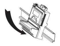
C. Slide base into position and lock rail clip. Be careful not to bend any pins.
