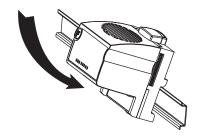
C. Slide module into position and lock rail clip.
