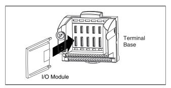
To remove a dual-channel module, squeeze the legs of the module together to unlock, then pull from the terminal base.
