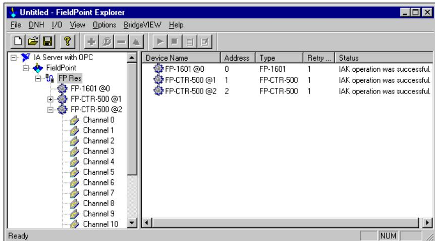
The hierarchy includes all of the modules connected to the FP-1601. The default name of each device found includes the name of the FieldPoint module, followed by a space, the @ sign, and the address of the module (for example, FP-1601 @0). For each module found, one I/O item is created for each channel on the module, and if all the channels are of the same type, one I/O Item is created to represent all the channels on that module collectively.
