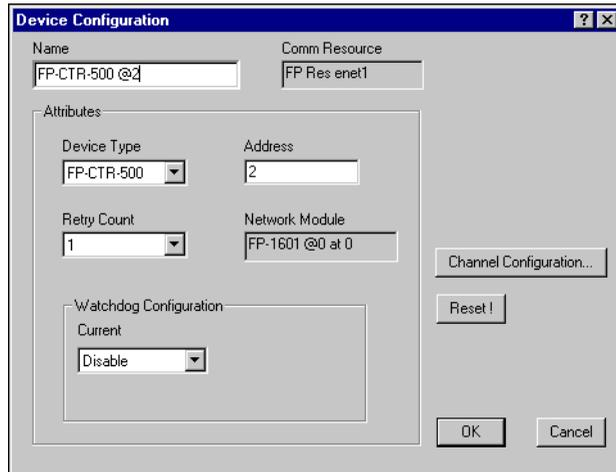
For output modules, you can choose settings for **Watchdog Configuration**. Refer to the [Guarding Against Network Failures \(Network Watchdog\)](#) section in Chapter 4, [Feature Set Description](#), for more information about the network watchdog feature.
