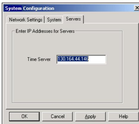
The **Time Server** is a networked computer that runs the NI Time Service. This is usually one of the computers that runs FieldPoint software. The FP-1601 has a battery-backed internal clock that provides accurate time stamps in the absence of a Time Server. However, the FP-1601 must contact a time server at least once to set the internal clock initially.
