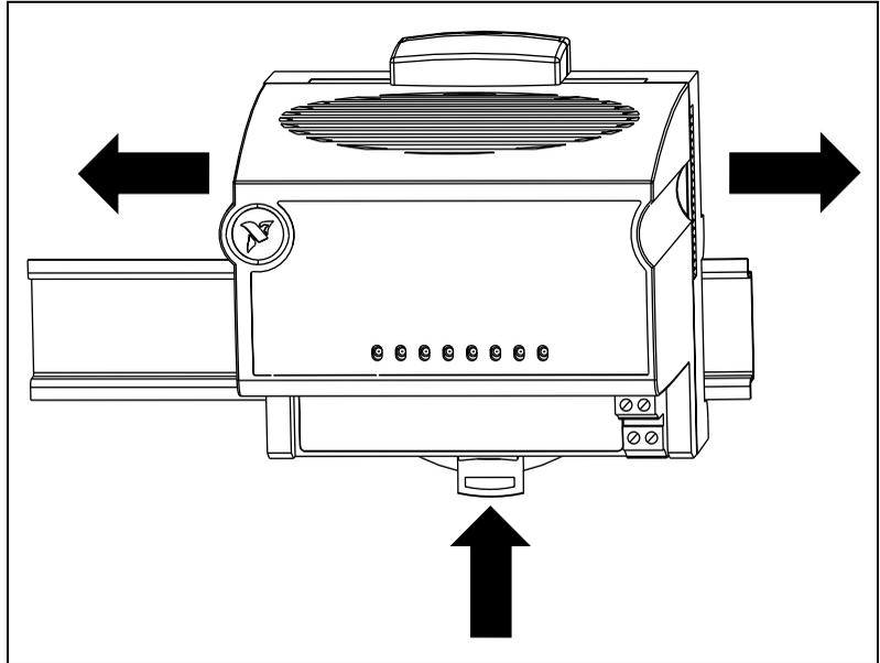
After the FP-1601 is mounted to the DIN rail, connect the terminal base to it.
