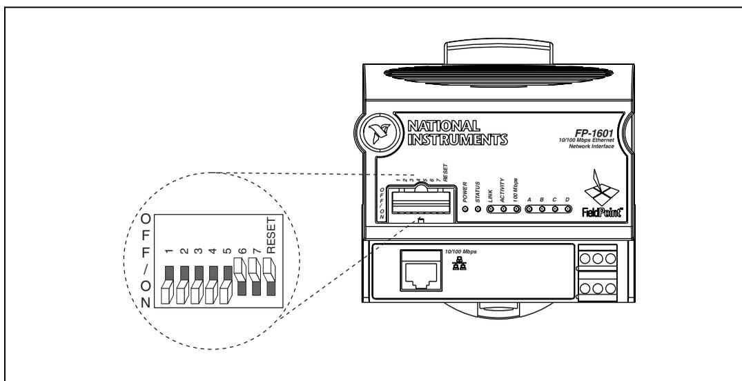
Switches 1, 2, 3, 4, 5, 6, and 7 are user-accessible DIP switches. They may be read by the FieldPoint LabVIEW VIs, but have no default functionality.
