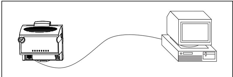
The host PC communicates to the FP-1601 over a standard Ethernet connection. If the host PC is already configured on a network, you must configure your FP-1601 on the same network. If neither is connected to a network, you can connect the two directly using a CAT-5 crossover cable. If you need to build your own cable, refer to Appendix D, *Specifications*, for more information about Ethernet cable wiring connections.
