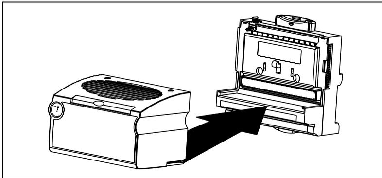
2. Firmly press the module onto the terminal base. The terminal base latch locks the I/O module into place when the ejector button pops up on top of the terminal base.
