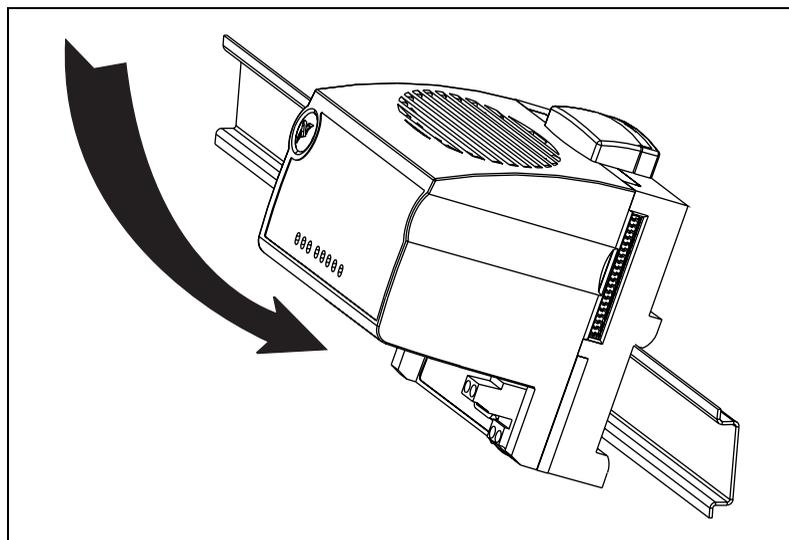
4. Slide the FP-1601 to the desired position along the DIN rail. After it is in position, lock it to the DIN rail by pushing the rail clip to the locked position, as shown in the following illustration.
