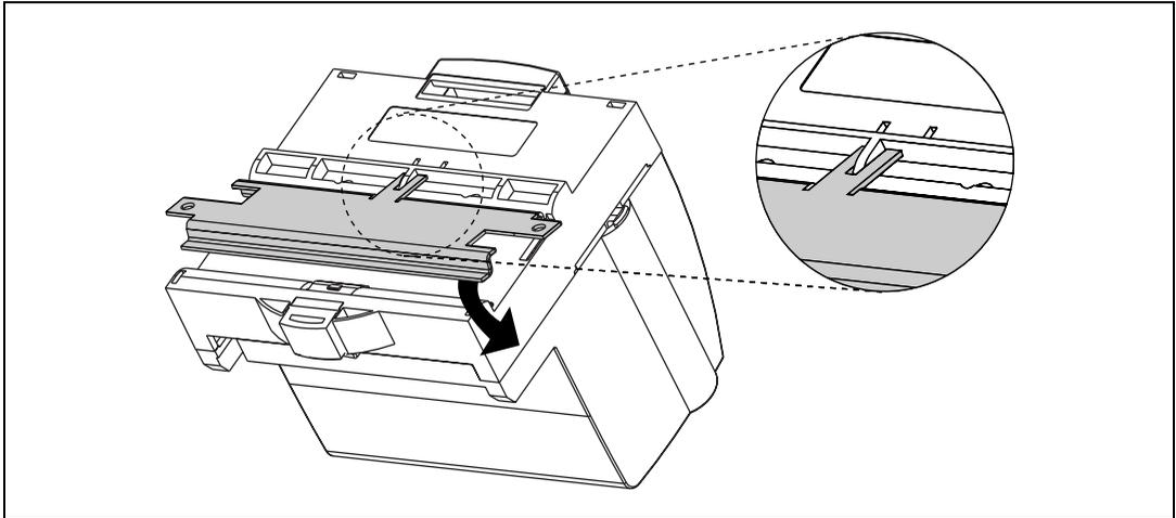
4. Lock the panel mount accessory into place by pushing the rail clip to the locked position.
