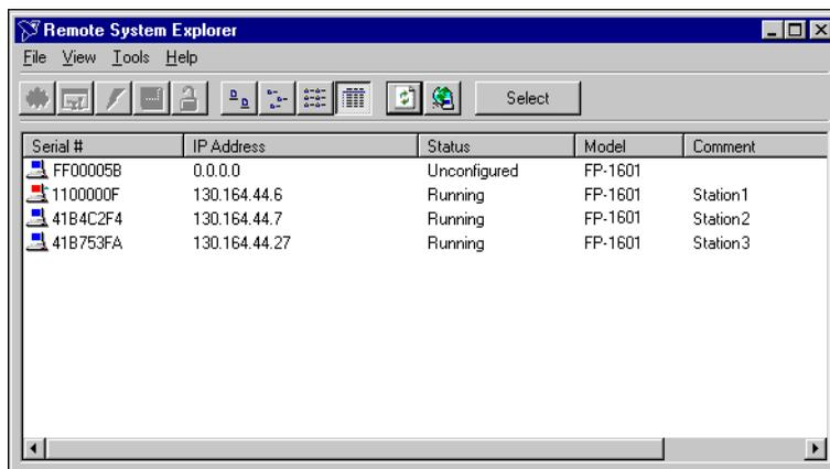
Remote System Explorer launches and searches for any FP-1601 or other NI Ethernet devices on the subnet. The serial number shown corresponds to the serial number of your FP-1601. The status of the module is `Unconfigured` because you have not yet set the IP address for it.
