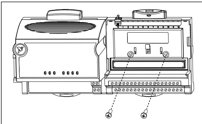
4. To add more terminal bases, repeat steps 1 through 3, mating the local bus connectors of each new terminal base to the connector of the last installed base. In most cases a single FP-1601 can support up to nine terminal bases, depending on the power consumption of the I/O modules. Refer to the [Wiring Power to Your FieldPoint System](#) section of this chapter for more information about power requirements.
