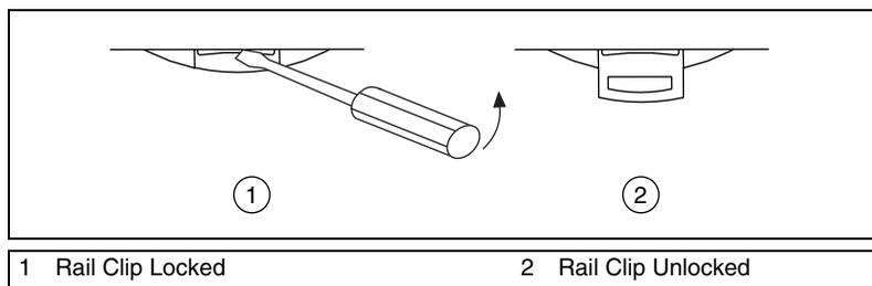
3. Hook the lip on the rear of the FP-1601 onto the top of a 35 mm DIN rail and press it down onto the DIN rail, as shown in the following illustration.
