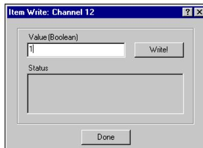
4. Enter the value you want to write in the **Value** field and click the **Write** button to write the value out. The value must be in the range of the channel that you configured in step 4 of the *Finding and Configuring*
