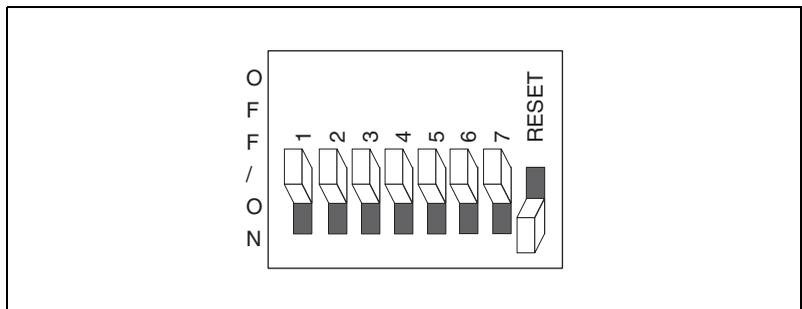
3. Power up the FP-1601 and wait for the red **STATUS** LED to start flashing. When it flashes, the FP-1601 is in reset mode.
