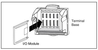
Figure 5. Installing a Dual-Channel Module in the Terminal Base
