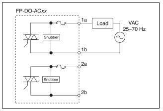
Figure 17. Signal Connections for Discrete AC Output Modules
