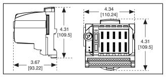
Figure 18. Mechanical Dimensions of the FP-TB-10
