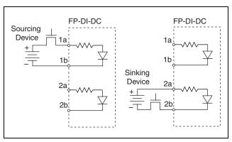
Figure 14. Connecting Sourcing and Sinking Devices to the FP-DI-DC
