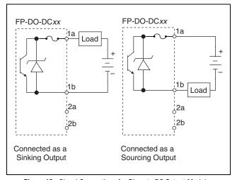
Figure 16. Signal Connections for Discrete DC Output Modules
