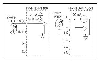
Figure 10. Two- and Three-Wire RTD Input Module Signal Connections
