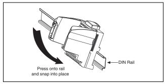
Figure 2. Mounting the Terminal Base on a DIN Rail
