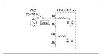
Figure 15. Wiring Diagram for Discrete AC Input Modules
