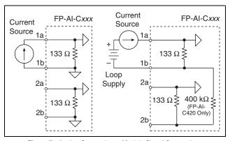
Figure 7. Analog Current Input Module Signal Connections
