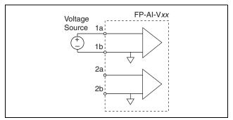
Figure 8. Analog Voltage Input Module Signal Connections
