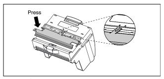
Figure 4. Snapping the Panel-Mount Accessory onto the Terminal Base
