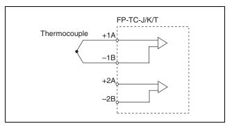
Figure 9. Thermocouple Input Module Signal Connections
