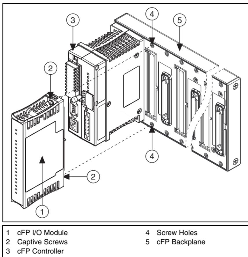
**Figure 2.** Installing the cFP-CTR-500
