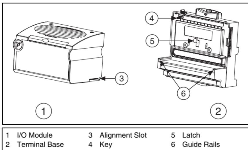
**Figure 1.** Installing the FP-CTR-500
