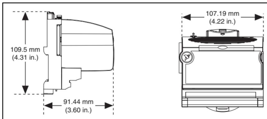
**Figure 12.** FP-CTR-500 Mechanical Dimensions
