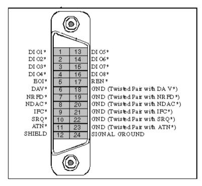
Figure C-1. GPIB Connector Showing Signal Assignment
