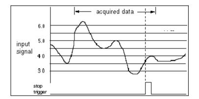
In the above illustration, **total scans to acquire** is 1000 and **pretrigger scans to acquire** is 900. The stop trigger can come from digital trigger A or an analog trigger (**trigger or pause condition** = 1: Trigger on rising edge or slope, **level** = 3.7, **window size** = 0.5).
