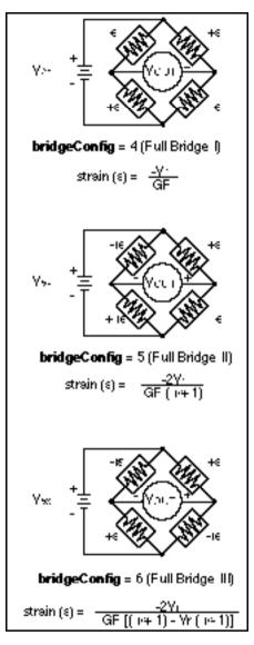
Figure 29-3. Strain Gauge Bridge Completion Networks (Full-Bridge Configuration)
