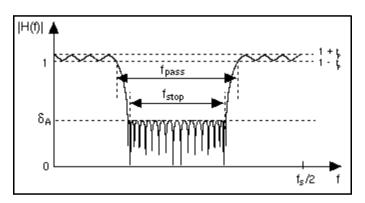
Figure 42-4. Bandstop Filter
