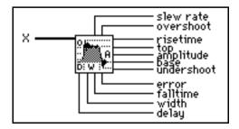
The waveform-related parameters are **slew rate**, **overshoot**, topline (**top**), **amplitude**, baseline (**base**), and **undershoot**. The time-related parameters are **risetime**, **falltime**, **width** (duration), and **delay**.
