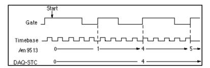
Figure 27-5. Unbuffered Mode 4 Rising-Edge Period Measurement
