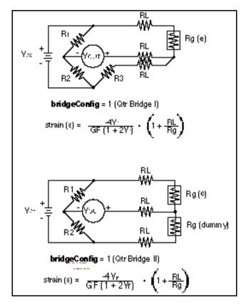
Figures 29-1 through 29-3 illustrate the bridge-completion networks available.
