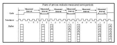
Figure 27-9. Buffered Mode 7 Semi-Period Measurement
