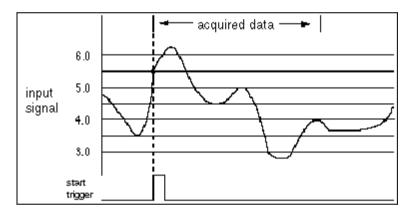
In the above illustration, **total scans to acquire** is 1000 and **pretrigger scans to acquire** is 0. The start trigger can come from digital trigger A or an analog trigger (**trigger or pause condition** =1: Trigger on a rising edge or slope, **level** = 5.5, **window size** = 0.2).
