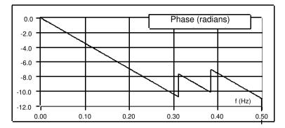
The discontinuities in the phase response arise from the discontinuities introduced when you compute the magnitude response using the absolute value. Notice that the discontinuities in phase are on the order of *pi*. The phase, however, is clearly linear. See Appendix D, *References*, for material that can give you more information on this topic.
