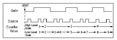
Figure 27-1. Unbuffered Mode 2 and 3 Counting
