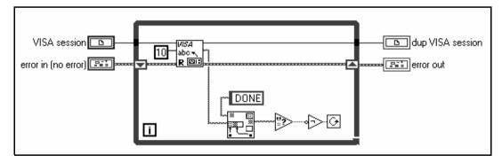
**Figure 32-2.** Incorrect Mechanism for Escaping from While Loop
