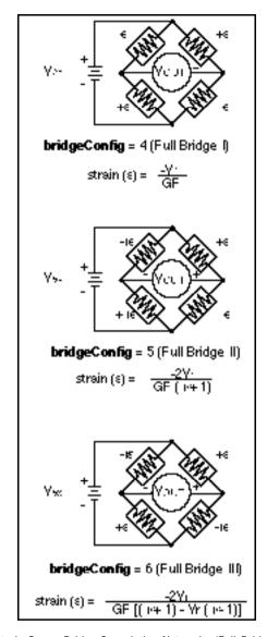
Figure 29-3. Strain Gauge Bridge Completion Networks (Full-Bridge Configuration)
