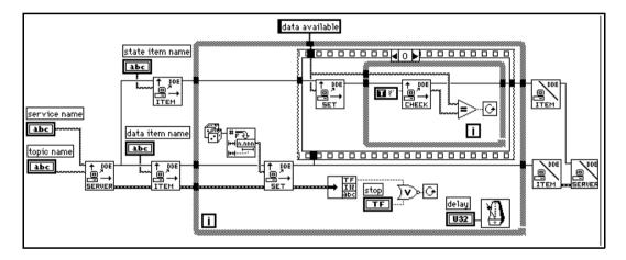
A client for this server, as shown in the following diagram, monitors the state item until it changes to *data available*. At that point, the client
