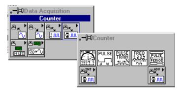
There are three classes of Counter VIs found in the **Counter** palette: the Easy, Intermediate, and Advanced Counter VIs. The following illustrates these VI classes.
