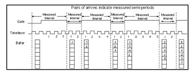
Figure 27-9. Buffered Mode 7 Semi-Period Measurement
