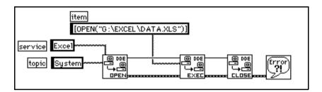
After you open a spreadsheet file, you can send commands to the spreadsheet to read cell values. In this case, your topic is the spreadsheet document name. The item is the name of a cell, a range of cells, or a named section of a spreadsheet. For example, in the following diagram LabVIEW can retrieve the value in the cell at row one column one. It then acquires a sample from the specified channel, and sends the resulting sample back to Excel.
