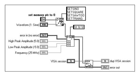
Figure 31-5. Tek VX4790 Config Std Wave Diagram
