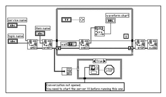
In the preceding diagram, LabVIEW opens a conversation. It then uses the DDE Advise Start VI to request notification of changes in the value of a data item. Every time through the loop, LabVIEW calls the DDE Advise Check VI, which waits for a data item to change its value. When the loop is finished, LabVIEW ends the advise loop by calling the DDE Advise Stop VI, and closing the conversation.
