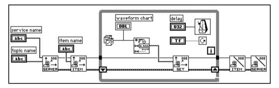
The VI in the preceding diagram registers a server with LabVIEW. The VI registers an item that it is willing to provide to clients. In the loop, the VI periodically sets the value of the item. As mentioned earlier, LabVIEW notifies other applications that data is available. When the loop is complete, the VI finishes by unregistering the item and unregistering the server.
