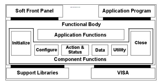
Figure 31-2. LabVIEW Instrument Driver Internal Design Model
