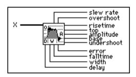
The waveform-related parameters are **slew rate**, **overshoot**, topline (**top**), **amplitude**, baseline (**base**), and **undershoot**. The time-related parameters are **risetime**, **falltime**, **width** (duration), and **delay**.
