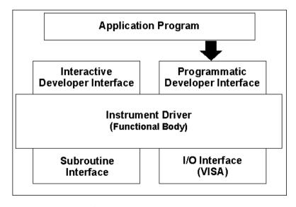
Figure 31-1. General Model of Instrument Drivers in LabVIEW
