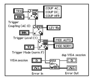
Figure 32-6. Simple Trigger VI without Programmatic Range Testing
