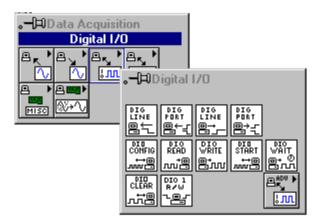
There are three classes of Digital I/O VIs found in the **Digital I/O** palette. The Easy Digital I/O VIs, Intermediate Digital I/O VIs, and Advanced Digital I/O VIs. The following illustrates these VI classes.
