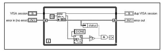
Figure 32-3. Correct Mechanism for Escaping from While Loop
