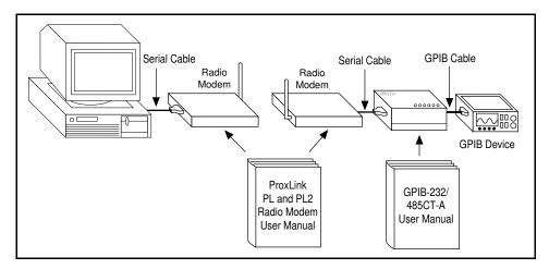
The *ProxLink PL and PL2 Radio Modem Family User's Manual* contains detailed information about the ProxLink PL2 radio modem. It includes instructions for serial port and radio parameter configuration.
