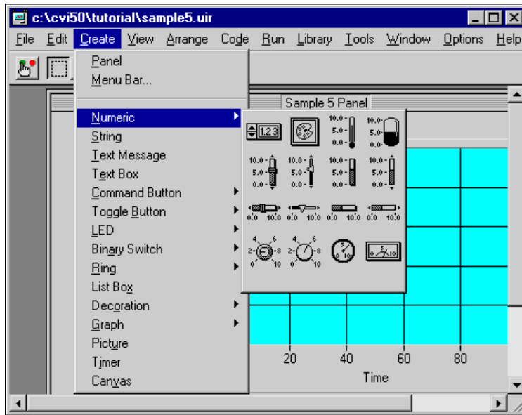
Figure 7-3. Selecting a Numeric Control from the Create Menu
