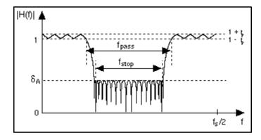
Figure 42-4. Bandstop Filter
