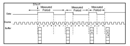
Figure 27-6. Buffered Mode 4 Rising-Edge Pulse Width Measurement
