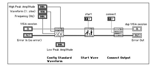
Figure 31-4. VIs in Tek VX4790 Example Diagram
