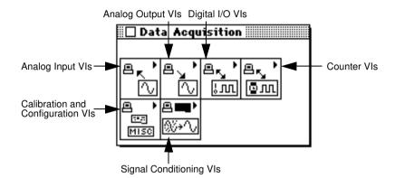
This section of the manual is organized in the order that the DAQ VI icons appear in the **Data Acquisition** palette from left to right. For example, in this section, the Analog Input VI chapters are followed by the Analog Output VI chapters, which are followed by the Digital I/O VI chapters, and so on. Most often, there are several chapters devoted to one class of DAQ VI in the palette, because many of the VI palettes also contain several subpalettes.
