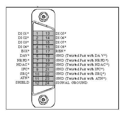
Figure C-1. GPIB Connector Showing Signal Assignment
