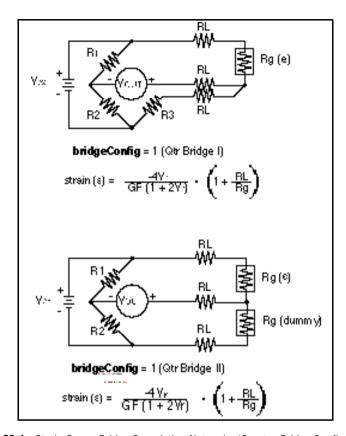
Figure 29-1. Strain Gauge Bridge Completion Networks (Quarter-Bridge Configuration)
