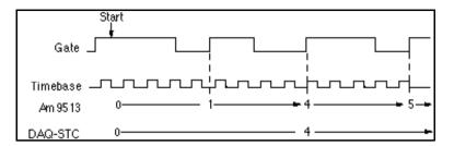
Figure 27-5. Unbuffered Mode 4 Rising-Edge Period Measurement
