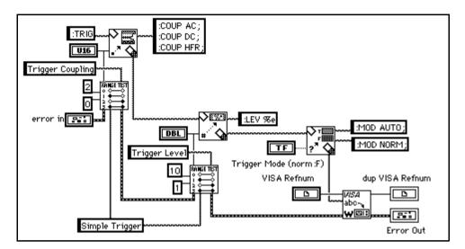
Figure 32-5. Simple Trigger VI with Programmatic Range Testing
