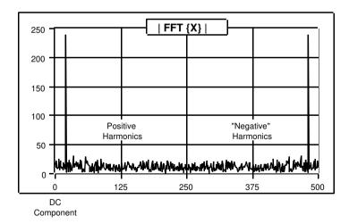
This format is an accepted standard in digital signal processing applications. It is convenient because it simplifies performing the inverse transform to obtain the final, processed result.
