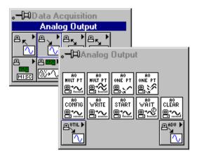
There are four classes of Analog Output VIs found in the **Analog Output** palette: the Easy Analog Output VIs, Intermediate Analog
