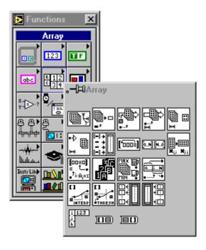
Some of the array functions are also available from the **Array Tools** palette of most terminal or wire pop-up menus. The illustration below shows the pop-up menu.
