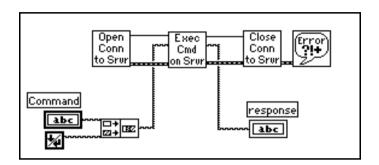
In the preceding diagram, LabVIEW first opens a connection to a server. It then sends a command to the server, gets a response back, and closes the connection to the server. Finally, it reports any errors that occurred during the communication process.
