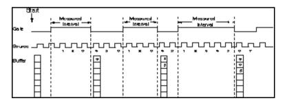
Figure 27-4. Buffered Mode 4 Rising-Edge Pulse Width Measurement
