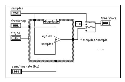
However, you may need to use frequency units of Hz (cycles/s). If you need to convert to Hz (or cycles/s) to cycles/sample, divide your frequency in cycles/s by the sampling rate given in samples/s. The following illustration shows an example of the Sine Wave VI generating a 60 Hz sine signal.
