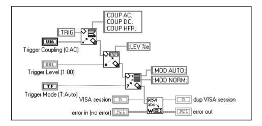
Figure 32-8. Simple Trigger Block Diagram
