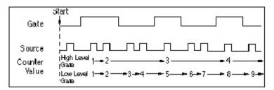
Figure 27-1. Unbuffered Mode 2 and 3 Counting
