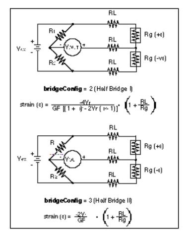
Figure 29-2. Strain Gauge Bridge Completion Networks (Half-Bridge Configuration)
