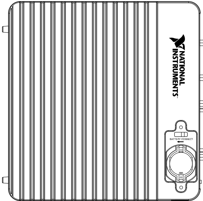
Figure 16. Side of Device with Removed Battery Cover Plate and BATTERY CONNECT Switch in Disconnected Position
