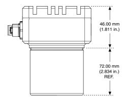
Figure 7. Side View with Dimensions
