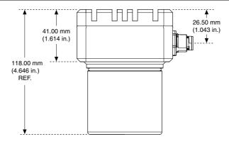
Figure 8. Bottom View with Dimensions
