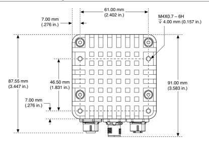
Figure 6. Side View with Dimensions
