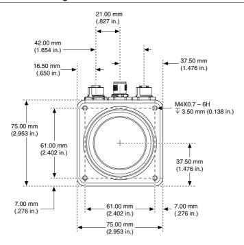
Figure 5. Back View with Dimensions
