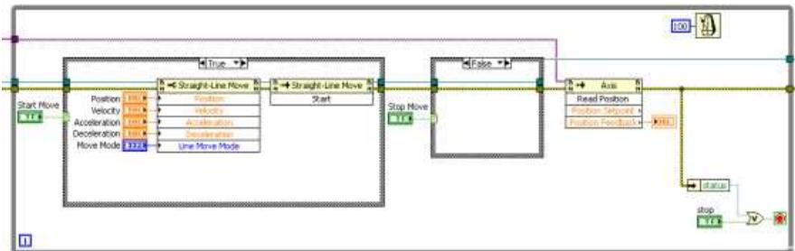
After the move has been stopped, errors are cleared and the motion reference is destroyed.
