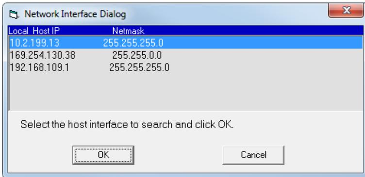
Normally, Drive Discovery only detects one network interface card (NIC), and selects it automatically. If you are using a laptop and have both wireless and wired network connections, a second NIC may appear. Please select the NIC that you use to connect to the network to which you’ve connected your device. Then click **OK**. Drive Discovery notifies you as soon as it has detected a device.
