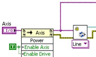
When the move is started, all of the configured parameters are written with a property node. The position feedback is read with an invoke node and displayed.
