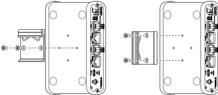
Clip the chassis onto the DIN rail with the larger lip of the DIN rail clip positioned up, as shown in the following figure.
