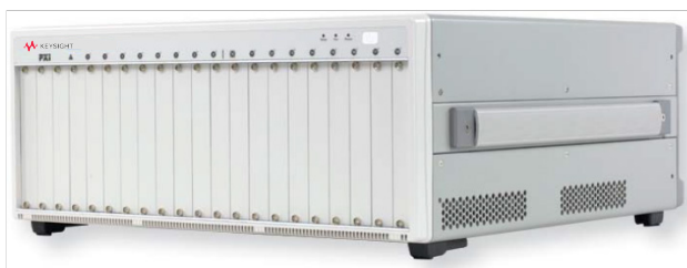
Figure 6. M9018A 18-slot chassis.
