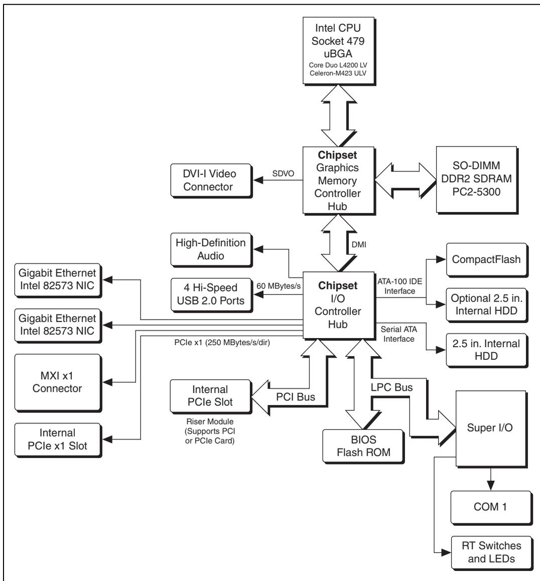
Figure 1-1. NI 3100/3110 Block Diagram
