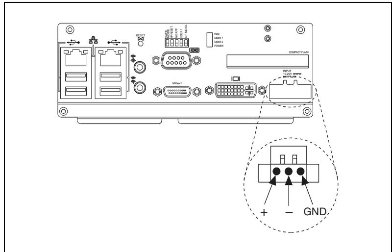
**Figure 3-9.** Power Connector Location and Pinout**Table 3-10.** Power Connector Signals
