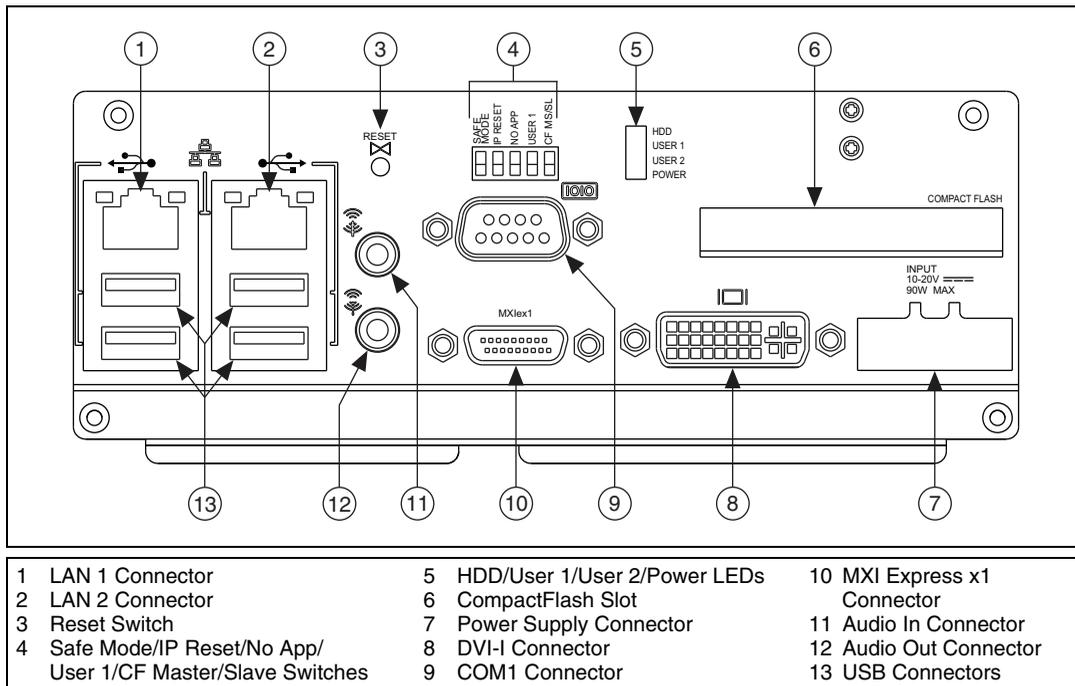
**Figure 3-1.** NI 3100/3110 Front Panel Layout
