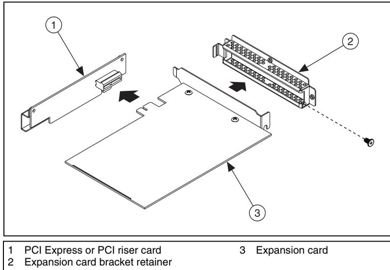
7. Mount the expansion card bracket to the retainer, as shown in the preceding figure. Be sure the card bracket is secured to the retainer by tightening the screw to  $0.31 \text{ N} \cdot \text{m}$  ( $2.7 \text{ lb} \cdot \text{in.}$ ) of torque.
