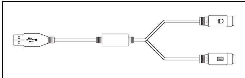
**Figure 4-1.** Y-Splitter Cable
