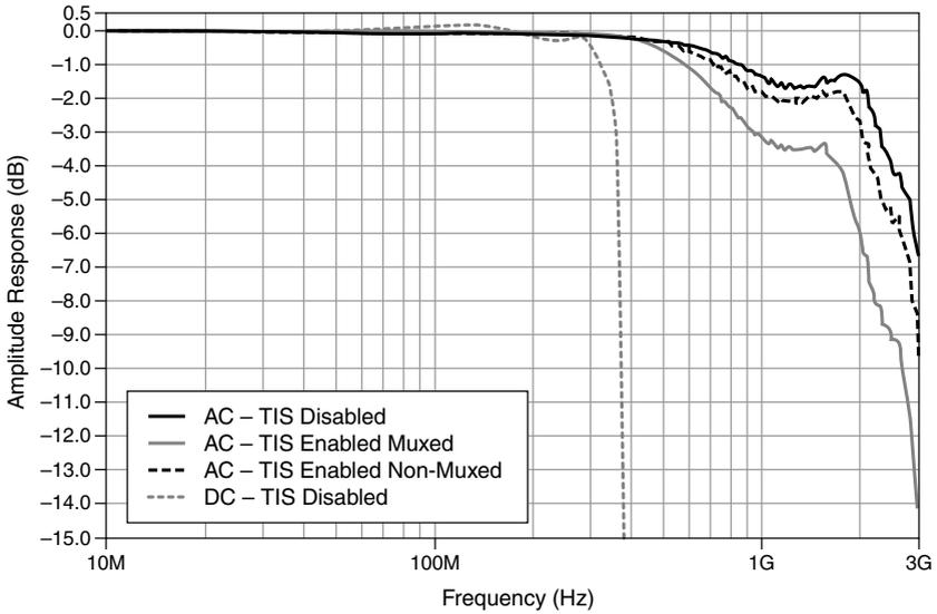
**Figure 13. DC Bandwidth (Referenced to Amplitude at 10 MHz)**
