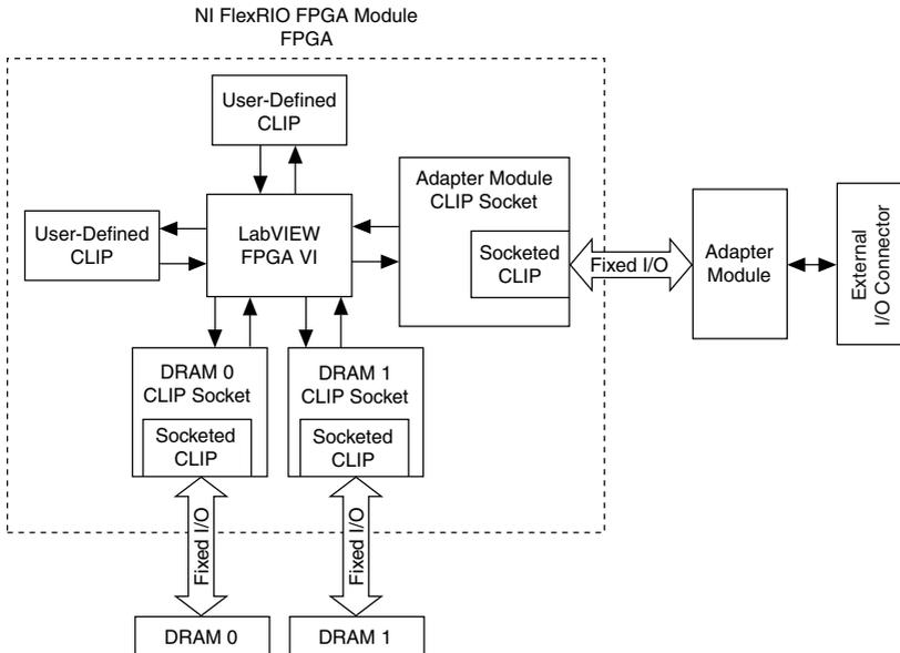
The NI 5772 ships with socketed CLIP items that add module I/O to the LabVIEW project.
