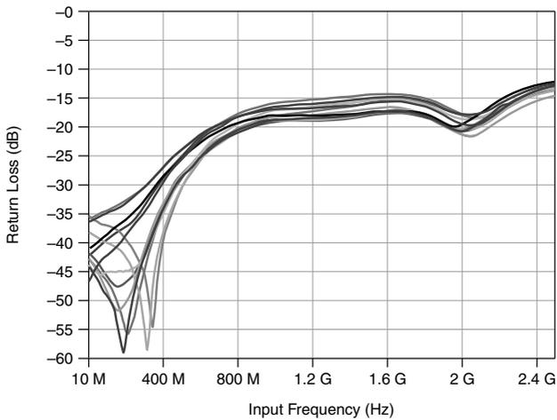
**Figure 10.** Analog Input VSWR (Multiple Channels Overlaid)
