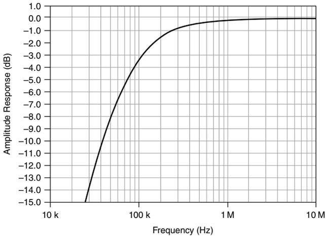
**Figure 12. High Frequency Response (Referenced to Amplitude at 10 MHz)**
