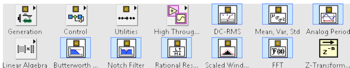
Figure 8. Just one of the palletes of FPGA IP included with LabVIEW FPGA.
