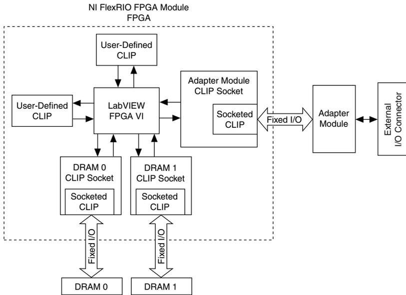
The NI 6581/6581B ships with socketed CLIP items that add module I/O to the LabVIEW project.
