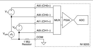
To connect floating differential signals to the NI 9205, you must connect the negative signal to COM through a 1  $M\Omega$  resistor to keep the voltage within the maximum working voltage. If the voltage source is outside the maximum working voltage, the NI 9205 does not read data accurately.
