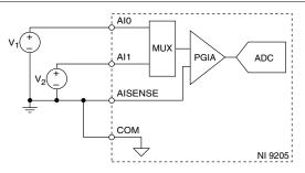
In an NRSE configuration, the NI 9205 measures each channel with respect to AISENSE. An NRSE configuration provides
