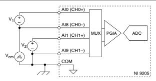
In a differential configuration, the NI 9205 rejects the common-mode noise voltage during the measurement of  $V_1$ . To connect grounded differential signals to the NI 9205, you must also connect the signal reference to COM.
