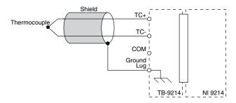
For most applications, you do not need to connect COM. Connecting to COM is not necessary for the following configurations:
