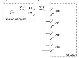
Configure function generator according to Table 5. 2.
