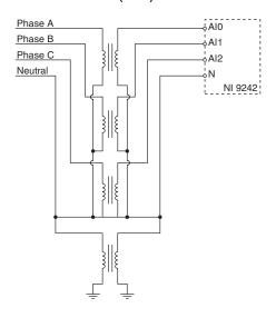
In a 4-wire WYE-to-WYE (full) configuration, the Neutral terminal on the NI 9242 measures the neutral-to-ground voltage through the bottom transformer. You can use a lower ratio transformer due to the typically low voltages on the Neutral terminal. Ensure that you scale each NI 9242 channel reading with the corresponding transformer ratio.
