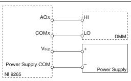
Figure 1. NI 9265 Current Accuracy Connections
