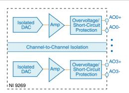
The analog output channels are floating with respect to earth ground and each other. Each channel has a digital-to-analog converter (DAC) that produces a voltage signal. Each channel
