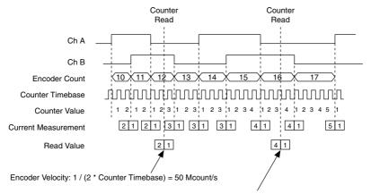
Encoder Velocity: 1 / (4 \* Counter Timebase) = 25 Mcount/s
