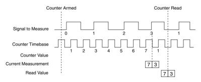
The following figure shows an example of Measurement Time.
