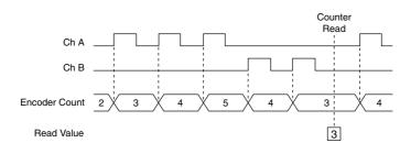
Figure 20. Two-Pulse Encoder Position Measurement
