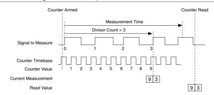
Figure 10. Divisor completes before Measurement Time
