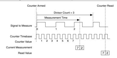
Figure 11. Measurement Time completes before Divisor
