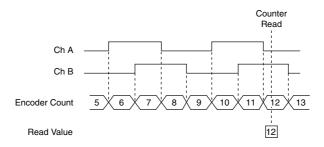
The following figure shows an example of Two-Pulse Encoder position measurement.
