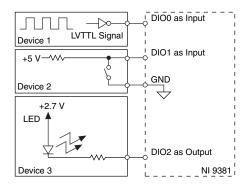
DIO channel direction is software selectable. Changing the direction on any channel does not affect the direction on the other channels.
