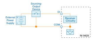
• The NI 9425 has sinking inputs. Sinking inputs provide a path to COM when the sourcing device connected to the NI 9425 drives current or applies voltage to DI.
