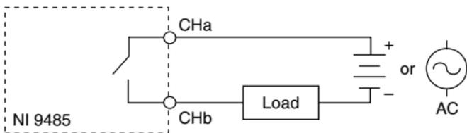
When the channel is turned on, the terminal connected to the load drives current or applies voltage to the load. When the channel is off, the terminal does not drive current or apply voltage to the load.
