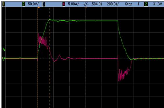
Figure 19. Current and Voltage Traces From Piezo IPhaseArray Configuration Example 1
