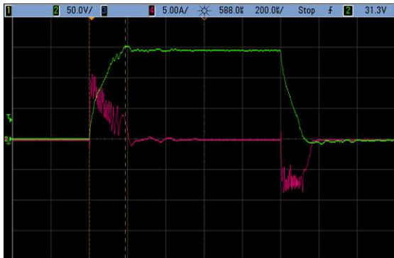
Figure 23. Current and Voltage Traces from Piezo IPhaseArray Configuration example 3
