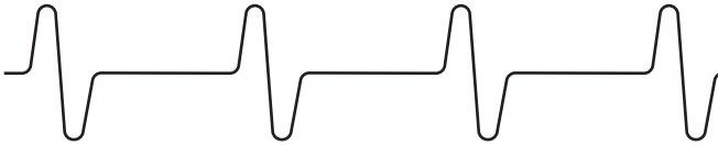
Figure 5. Incorrect Signal Polarity for VR Input Circuit
