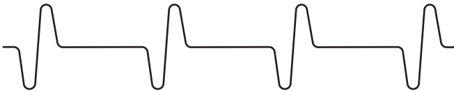
Figure 5. Incorrect Signal Polarity for VR Input Circuit
