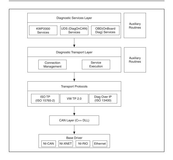
The Automotive Diagnostic Command Set is structured into three layers of functionality:
