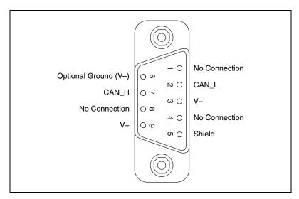
Figure 4-1. Pinout for 9-Pin D-SUB Connector
