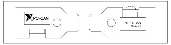
Figure 1-3. NI PCI-CAN Hardware Series 1 and 2 Labels
