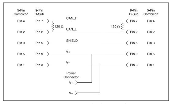
Figure 4-4. Cable Connecting Two CAN Devices
