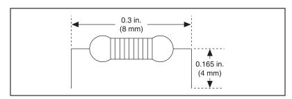
Figure 4-9. Preparing Lead Wires of Replacement Resistors
