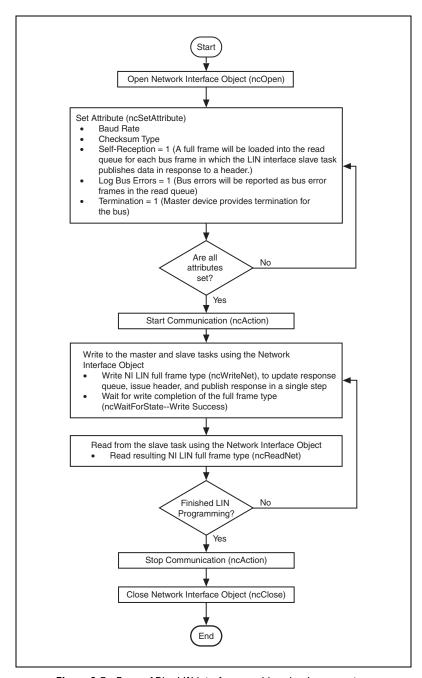
Figure 9-5. Frame API – LIN interface provides simple access to a single slave device that subscribes to data
