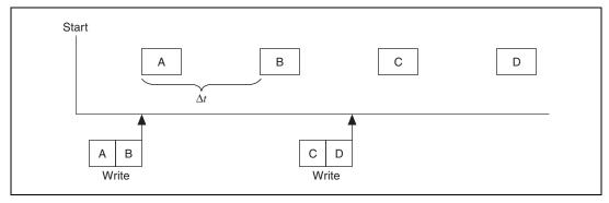
Figure 6-7. Example of Write with Sample Rate > 0, Output Mode
