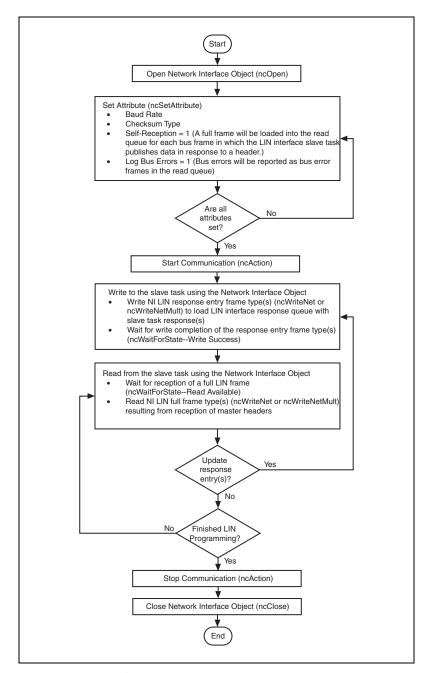
**Figure 9-4.** Frame API – LIN interface acting as slave
