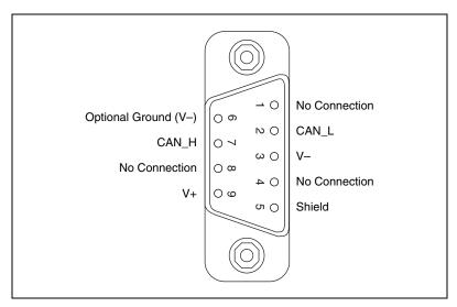
Figure 4-5. Pinout for 9-Pin D-SUB Connector
