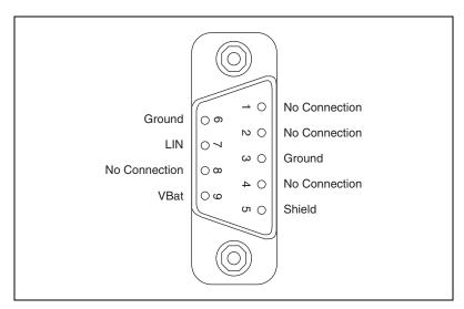
Figure 4-19. Pinout for 9-Pin D-SUB Connector
