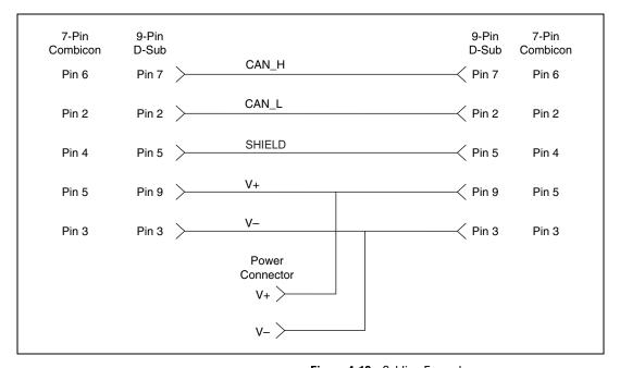
Figure 4-13. Cabling Example
