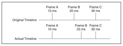
Figure 11-14. Example with Time Recovery Enabled
