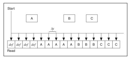
**Figure 6-4.** Example of Read with sample rate > 0
