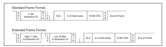
Figure B-2. Standard and Extended Frame Formats
