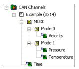
Figure 6-11. Mode Dependent Channels in the MAX Configuration Tree
