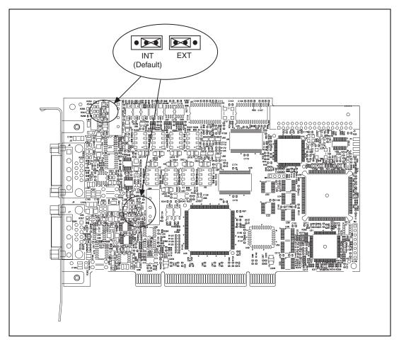
Figure 3-1. High-Speed VBAT Jumper Settings
