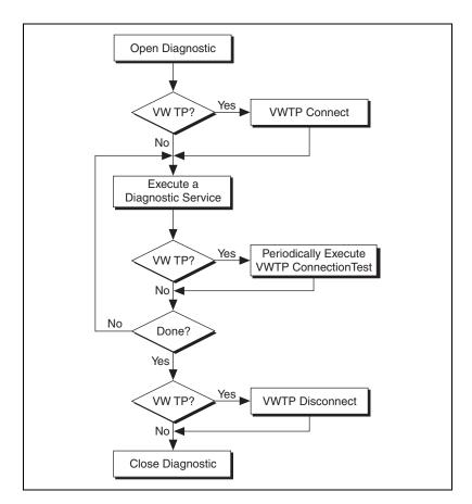
First, you must open a diagnostic communication link. This involves initializing the CAN/LIN port and defining communication parameters such as the baud rate. For CAN-based diagnostics, the CAN identifiers on which the diagnostic communication takes place must be defined also. No actual communication to the ECU takes place at this stage.
