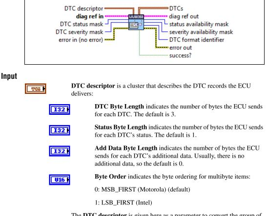
The **DTC descriptor** is given here as a parameter to convert the group of DTC parameters to a binary representation according to **DTC Byte Length** and **Byte Order**.
