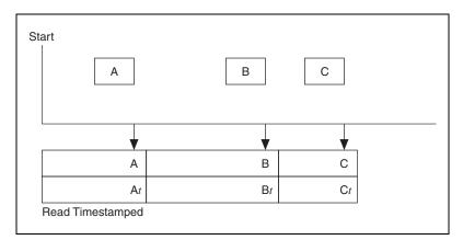
Figure 6-5. Example of Read Timestamped
