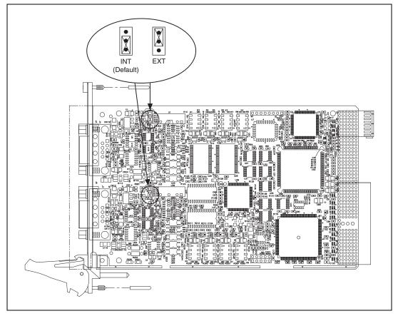
Figure 3-5. Low-Speed/Fault-Tolerant VBAT Jumper Settings
