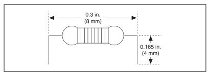
Figure 4-11. Preparing Lead Wires of Replacement Resistors
