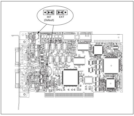
Figure 3-2. Low-Speed/Fault-Tolerant VBAT Jumper Settings
