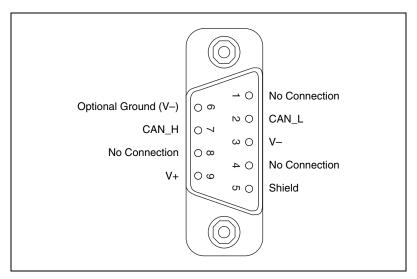
Figure 4-5. Pinout for 9-Pin D-SUB Connector
