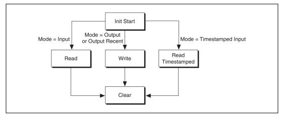
Figure 6-2. Basic Programming Model for Channel API
