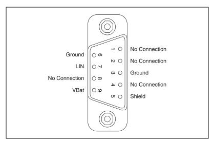
Figure 4-19. Pinout for 9-Pin D-SUB Connector
