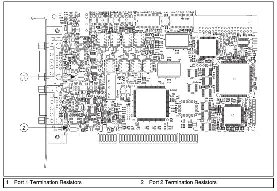
Figure 4-8. Location of Termination Resistors on PCI-CAN/LS2 Card
