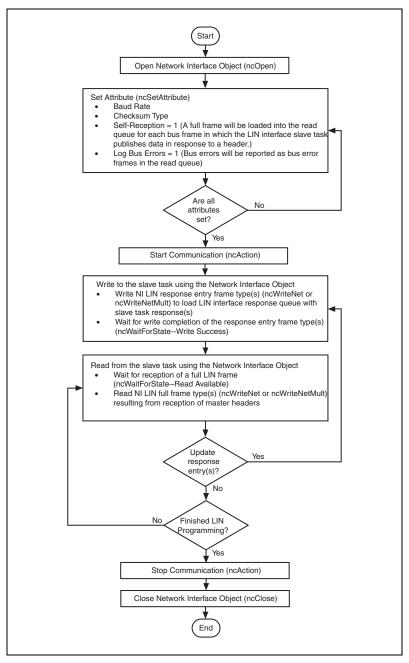
Figure 9-4. Frame API – LIN interface acting as slave
