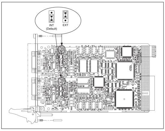
Figure 3-4. High-Speed VBAT Jumper Settings
