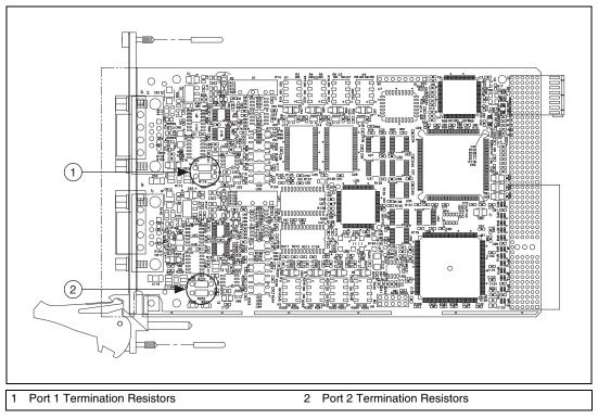
Figure 4-10. Location of Termination Resistors on a PXI-8460
