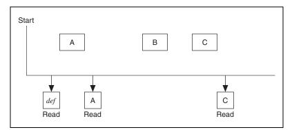
Figure 6-3. Example of Read with sample rate = 0
