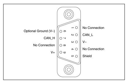
Figure 4-14. Pinout for 9-Pin D-SUB Connector
