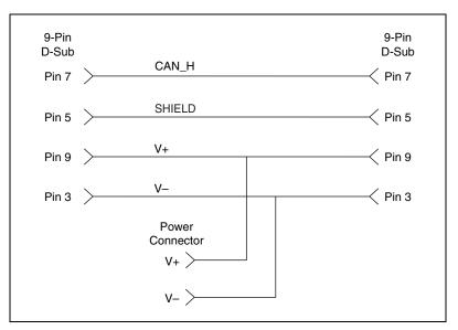
Figure 4-16. Cabling Example
