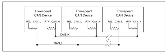
Figure 4-7. Termination Resistor Placement for Low-Speed CAN
