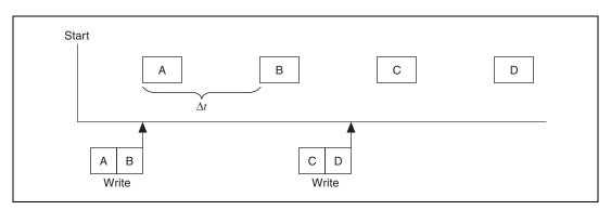
Figure 6-7. Example of Write with Sample Rate > 0, Output Mode
