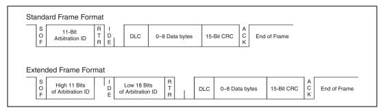
Figure B-2. Standard and Extended Frame Formats
