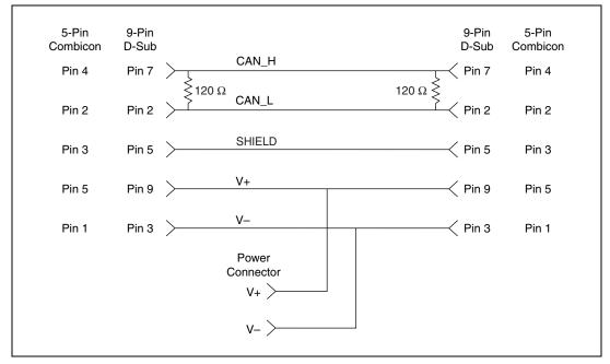
Figure 4-4. Cable Connecting Two CAN Devices
