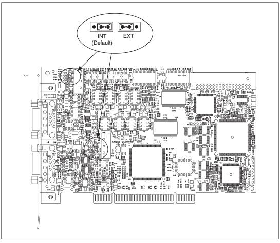
Figure 3-1. High-Speed VBAT Jumper Settings
