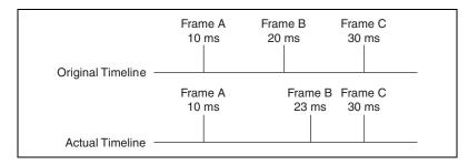
Figure 10-10. Example with Time Recovery Enabled
