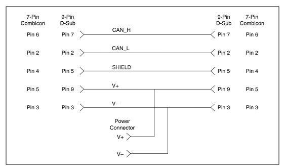
Figure 4-13. Cabling Example
