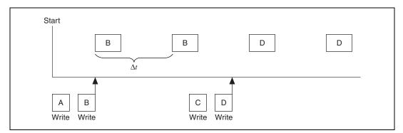
Figure 6-8. Example of Write with Sample Rate > 0, Output Recent Mode
