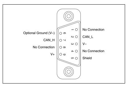
Figure 4-1. Pinout for 9-Pin D-SUB Connector
