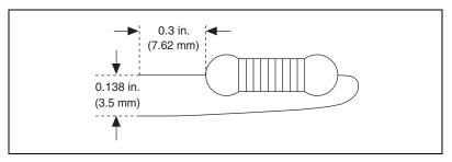
Figure 4-12. Preparing Lead Wires of PCMCIA-CAN/LS Cable Replacement Resistors
