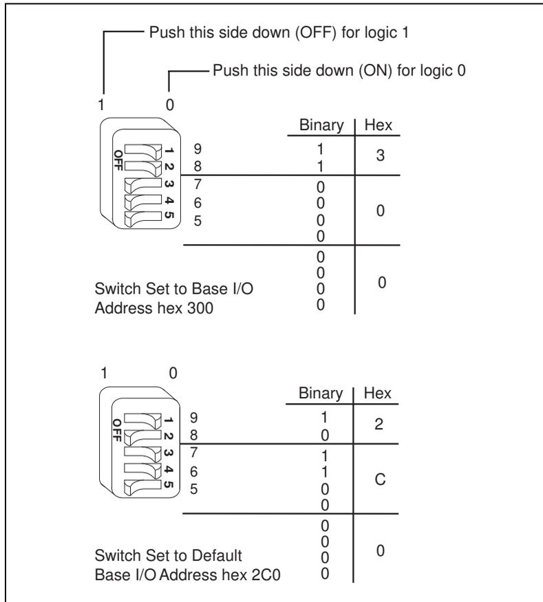
Figure 2-3. Base I/O Address Switch Settings
