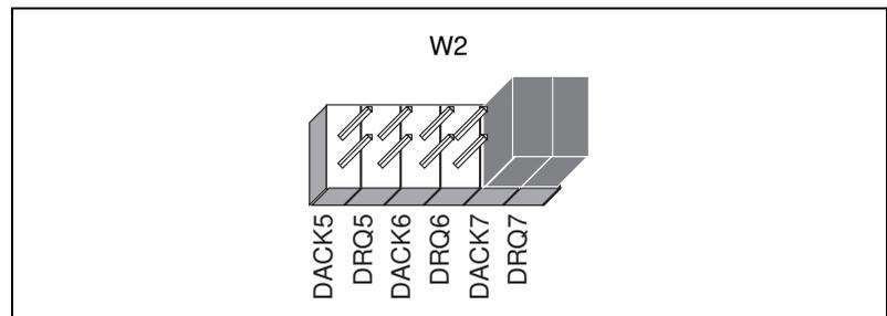
**Figure 2-6.** DMA Channel Jumper Setting for DMA Channel 7
