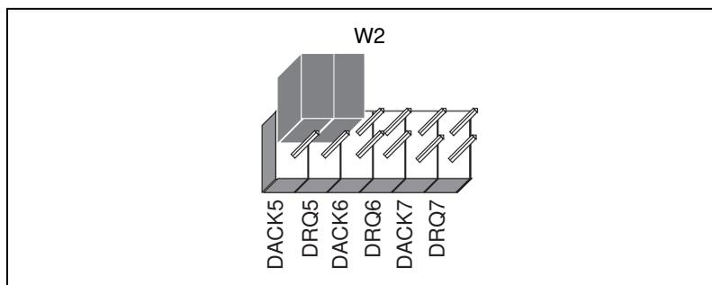
Figure 2-7. DMA Jumper Setting for No DMA Channel
