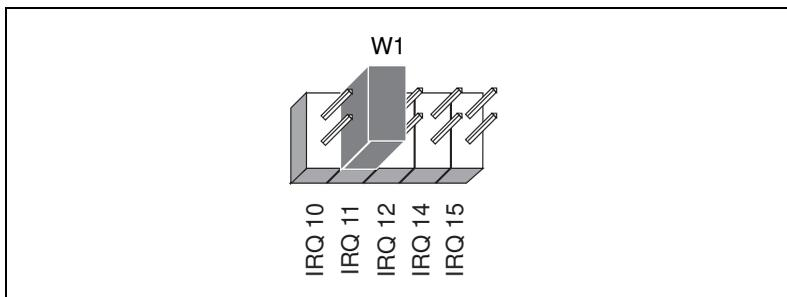
**Figure 2-4.** Interrupt Jumper Setting for IRQ11 (Default Setting)
