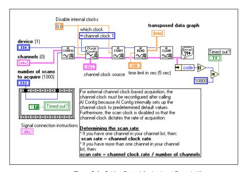
Figure 9-4. Getting Started Analog Input Example VI
