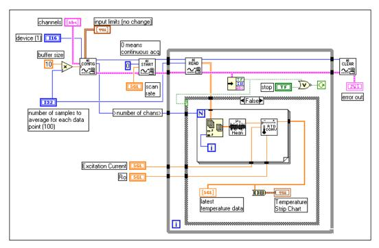
Figure 21-6. Measuring Temperature Using the Convert RTD Reading VI
