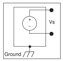
Figure 5-3. Floating Signal Sources
