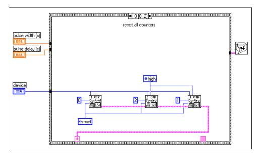
Figure 24-9. Frame 0 of Delayed Pulse (8253) VI
